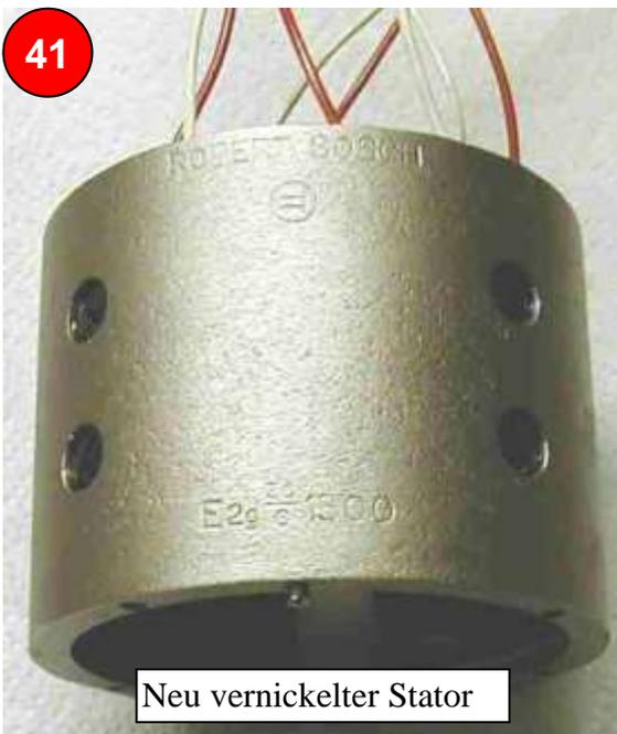
Neu vernickelter Stator
